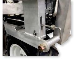
To secure the turret, a single control handle moves in and out keeping it from turning. When not attached to a tank it is necessary to lock the turret when moving to and from a tank. Unlocking the turret when attached to a tank allows for a 360° turning radius.
