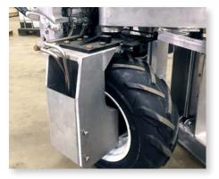
The parking brake interrupts the flow of hydraulic fluid to the orbital motor and locks the drive wheel in place. The parking brake should be used when connecting the dolly to a tank and for transporting on a utility trailer.
