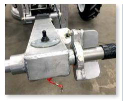
Forward and reverse is accomplished utilizing a single thumb control located on the handle bar. The up and down positions of the power unit forks are hydraulically controlled using a single toggle switch within easy reach of the operator. The handle bar is spring loaded, allowing the entire steering handle assembly to automatically return to the up position, keeping it out of the way when connecting to a tank.
