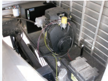
Optional self-contained 38 HP Kohler EFI power pack is protected from the elements neatly under the rear slope of the trailer.
