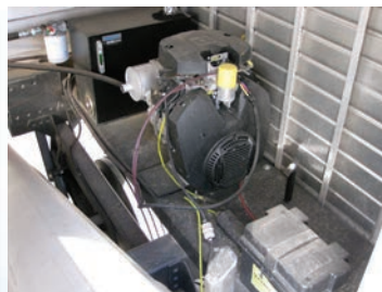
Optional self-contained 38 HP Kohler EFI power pack is protected from the elements neatly under the rear slope of the trailer.
