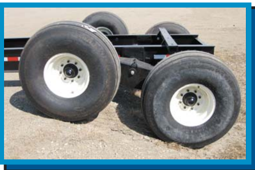
WALKING TANDEM REAR AXLE FOR ADDITIONAL STABILITY ON UNEVEN TERRAIN
